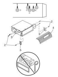
Fastening the unit to the factory radio mounting bracket.
